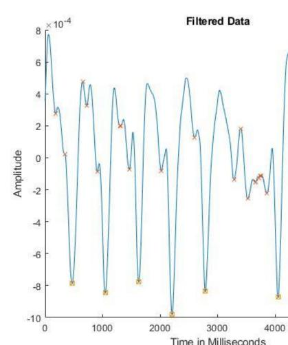
We exported data from the Labview Workbench where we were storing data generated by the sensor and imported it into Matlab to perform peak anaylsis to generate heart beat. From the data we compared our results with a commercial device to see if our results we gathered were in an acceptable range.
