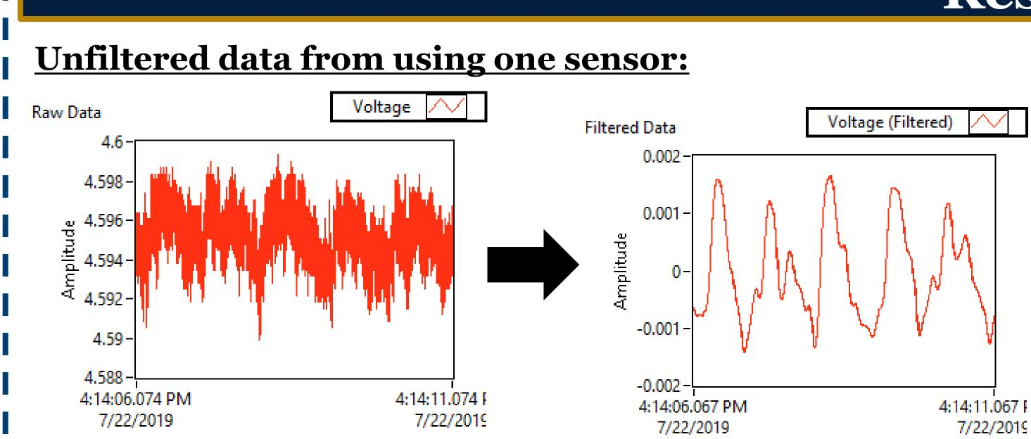
The figure on the left shows the raw data generated from our sensor and the figure on the right shows what that data looks like after it has been passed through the bandpass filter. From this data we were able to program our sensor to give us a readout of the beats per minute made • by the heart.
