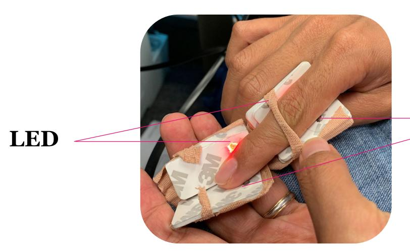
Shown above is a picture of the device we prototyped. By using two sensors at different distances along the same finger we were able to see heart rate variability from the data produced
