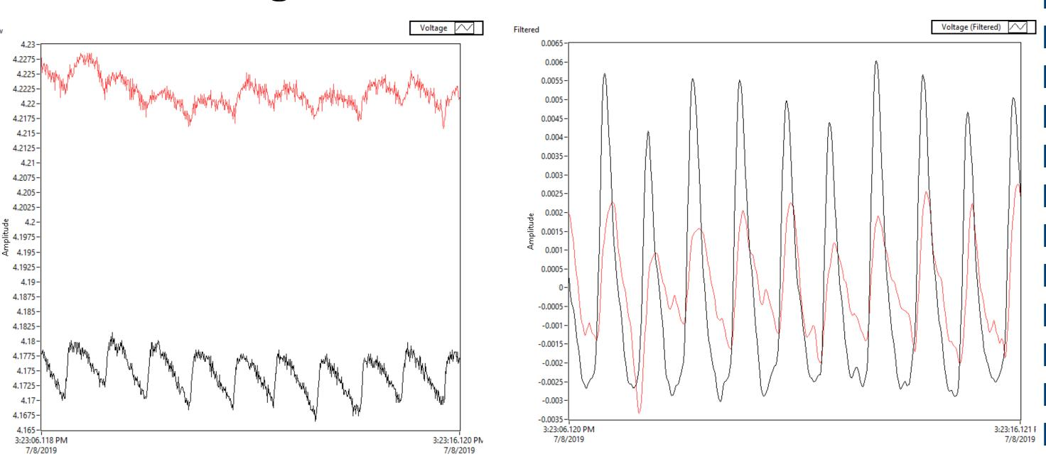
We prototyped two different sensor designs to generate two PPG signals and found that two LEDs and two photoresistors along the finger gave the best signal. Using a bandpass filter for the data generated and adjusting the millisecond differences between the sensors we were able to produce two waves that flow alongside one another.
