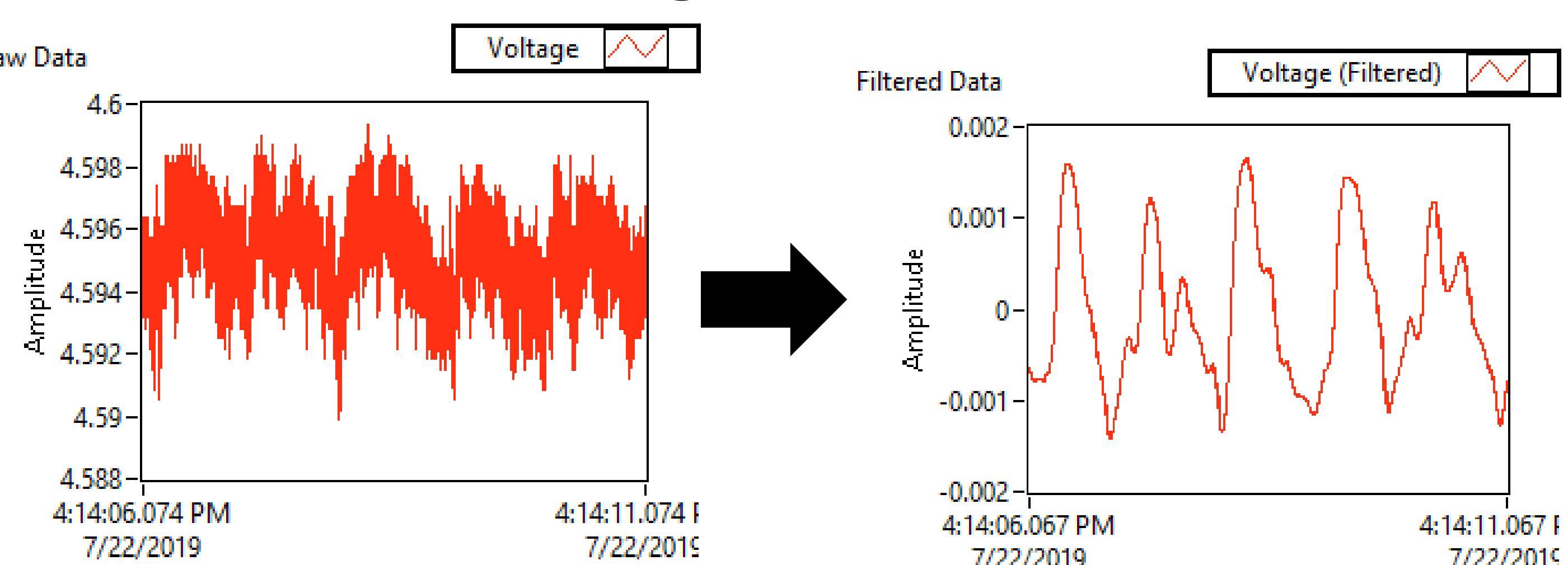
The figure on the left shows the raw data generated from our sensor and the figure on the right shows what that data looks like after it has been passed through the bandpass filter. From this data we were able to program our sensor to give us a readout of the beats per minute made by the heart.
