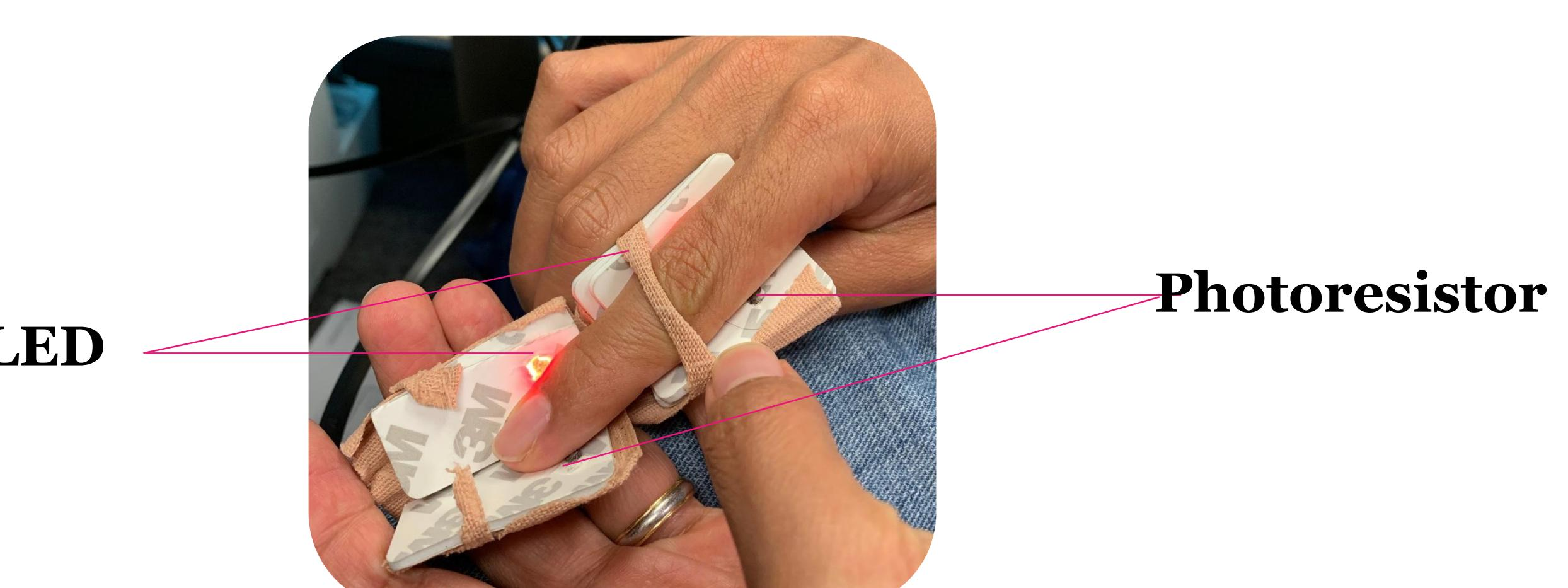
Shown above is a picture of the device we prototyped. By using two sensors at different distances along the same finger we were able to see heart rate variability from the data produced
